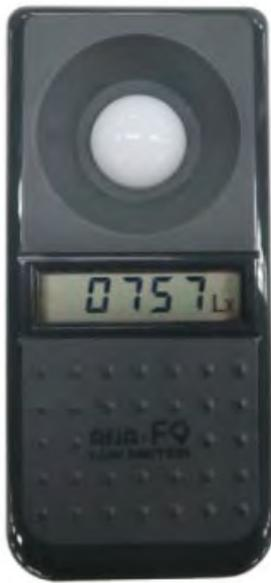
The white hemisphere of this illuminometer senses light, and a value is displayed on the monitor.
