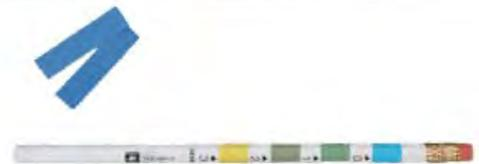
A-D Strips are made of blue paper that changes color when exposed to acid. The extent of the deterioration can be judged by comparing the color of the exposed A-D Strip with the color swatches on the indicator pencil.
