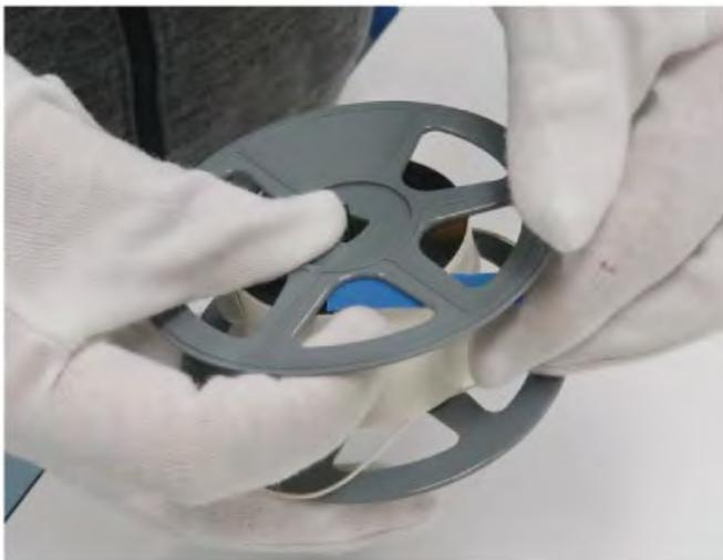
A blue A-D Strip is inserted between the microfilm and the reel so that it touches the film.
