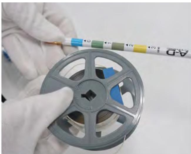
After 96 hours, the color of the A-D Strip is compared with the color swatches. A yellow strip indicates that significant levels of acidity were detected.
