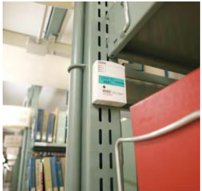
To measure temperature and humidity, place a data logger in a stack for a certain period of time.
