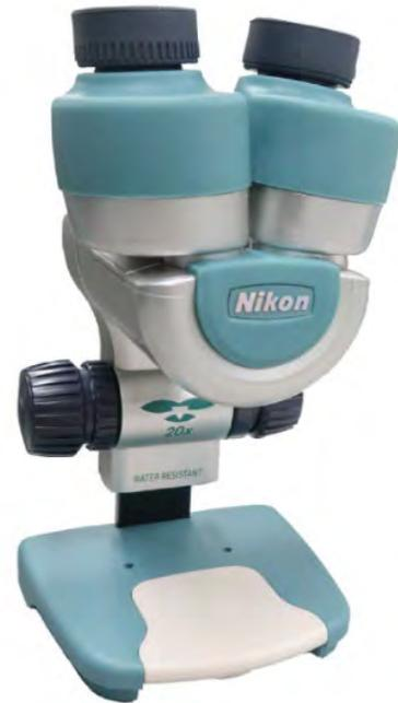
When pests are found to be infesting library materials, an overall improvement of the storage environment is called for<sup>1</sup>. The stereomicroscope shown here is used to identify small insects and their traces that cannot be seen with the naked eye.
