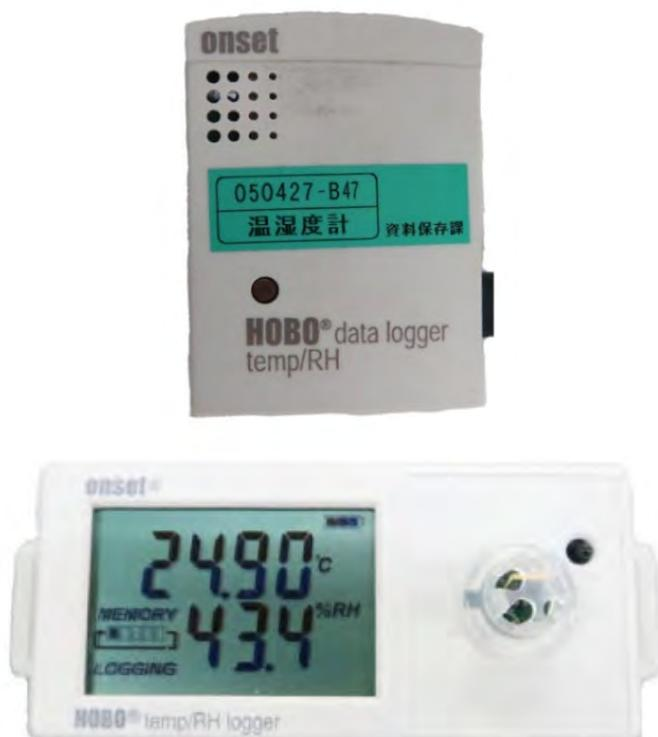
Ensuring that library materials remain available for long-term use requires that they be stored at an appropriate temperature and humidity in order to prevent damage and deterioration. Ordinary paper materials should ideally be stored at a temperature of 22°C and a relative humidity of 55%.
