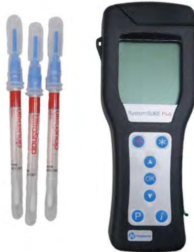
The equipment shown here can quickly quantify the amount of adenosine triphosphate (ATP), which is a biologically derived substance. If the amount of ATP contained in dirt found in books or on bookshelves is high, we determine that the dirt is of biological origin and treat it as active mold. Mold is a significant threat to library materials, and treatments such as book cleaning and fumigation are needed to remove and annihilate it.
