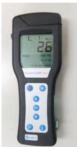
The result appears in 15 seconds. The decision on whether anti-mold treatment is necessary is made based on the test results and the overall condition of the library materials.
