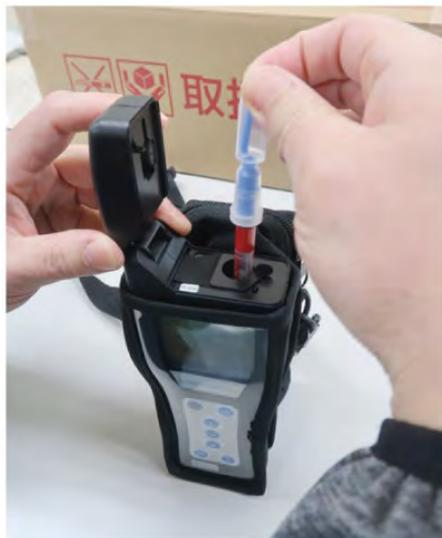
Immediately place the test tube in the luminometer.
