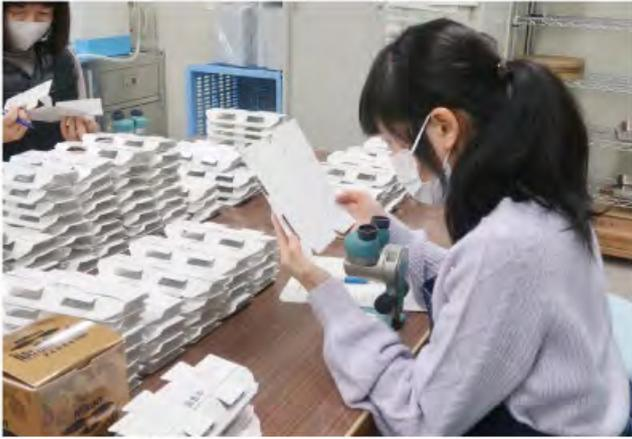
First we perform a naked-eye inspection of the inside of the traps.
